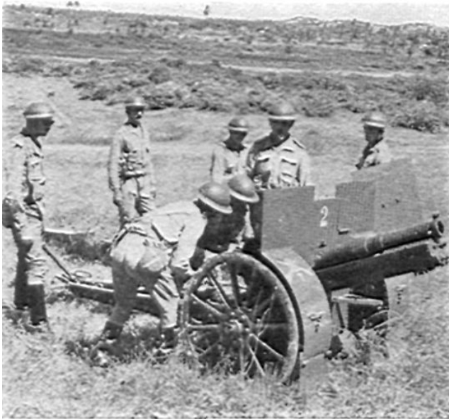
Brazil's pack artillery is armed with the 75-mm Schneider. 18.6 calibers long.
