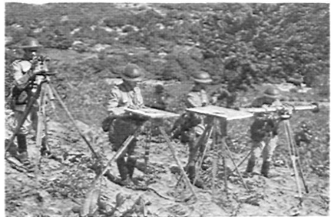
Fire control equipment includes a Zeiss range finder of familiar pattern. At the left is a "circulo de visada," an azimuth-measuring device onto which is clamped a pair of binoculars to furnish the optical portion of the instrument.
